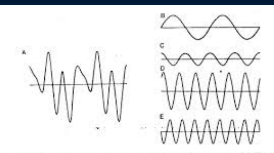
Fig. 1. The wave form A, a complex tone, is in fact the sum of the simple same B-E. This is an illustration of Fourier's theorem that every vibration of frequency f can be analyzed mathematically into a series of sinusoidal vibrations with frequencies f. 2f. 3f. etc. These sinusoidal vibrations are called the httmsin's
