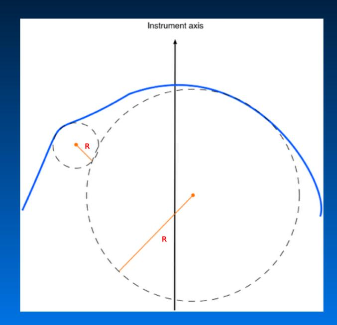
$$R = \left| \frac{\left(1 + {y'}^2\right)^{3/2}}{y''} \right|, \quad \text{where} \quad y' = \frac{dy}{dx}, \quad y'' = \frac{d^2y}{dx^2},$$
